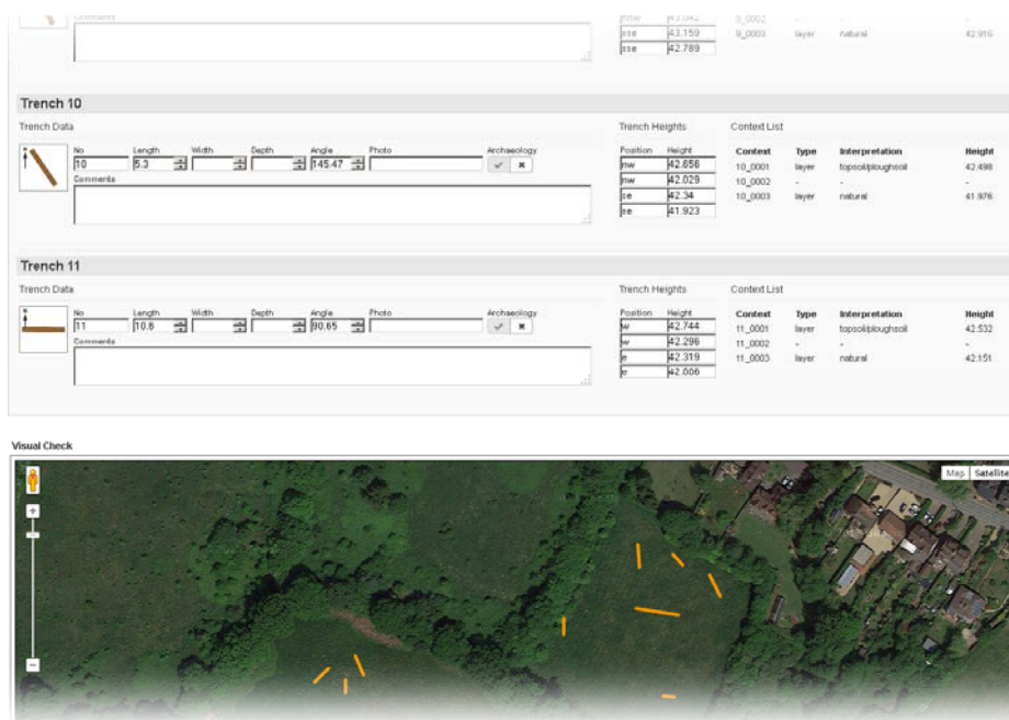
Figure 14. Extract of trench register form showing calculated dimensions and orientations, and map view of survey data
